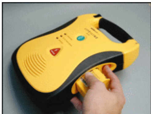
Figure 1 – Press the orange release button to eject the battery pack from the AED.
